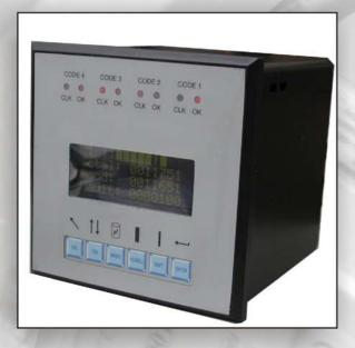
The rather intuitive user interface installed in the system enables the operator to visualise and control several codes at the same time. The wide variety of functions and options available in the software guarantee excellent code reading results in every condition.
